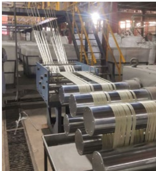
Manufacturing Polyester Staple Fiber (PSF) from waste PET bottles
